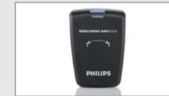
The **AirBridge** receiver module communicates with the SpeechMike Air from up to 10 meters away.
